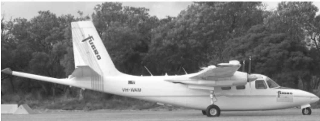
Specially equipped aeroplane for magnetic surveys (courtesy Fugro)
